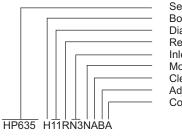
Series - Regulator Base Model Body/Bonnet/Trim Diaphragm/Main Valve Seat Relieving Options Inlet/Outlet Ports Mounting Cleaning Options Adjustment Selections Control Range Settings
