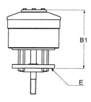
Actuator with top mounted positioner
