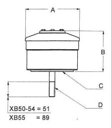
On-Off actuator - With spacer-bars
